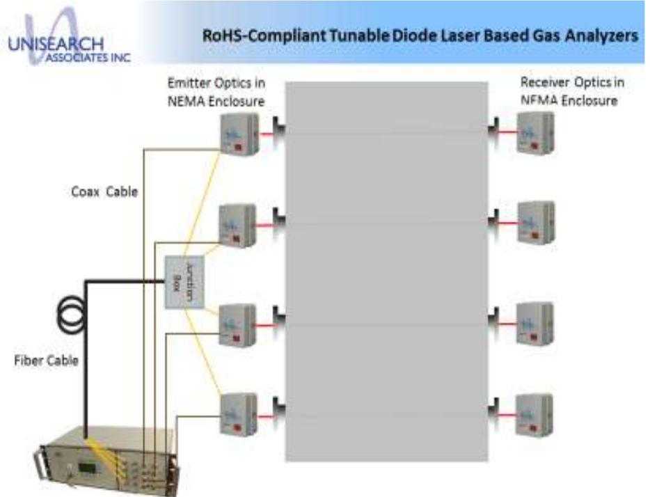
*Schematic of the in-situ monitor heads for continuous measurement of HCL*
