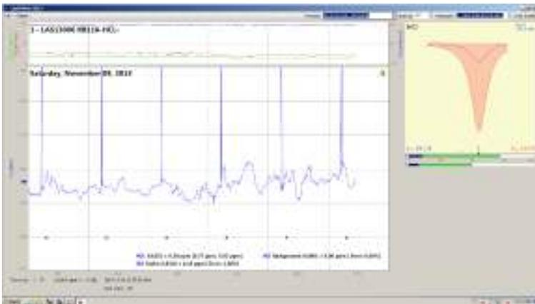
*HCl measurements in the stack emissions of a coal-fired power plant*
